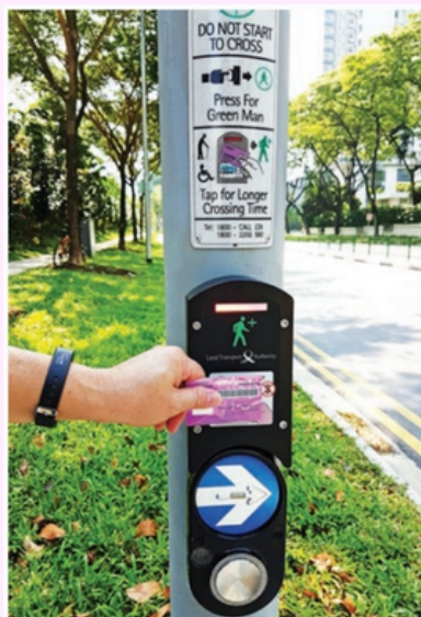
By tapping their EZ-Link cards at Green Man+ traffic light posts, the elderly or pedestrians with disabilities get more time to cross roads
