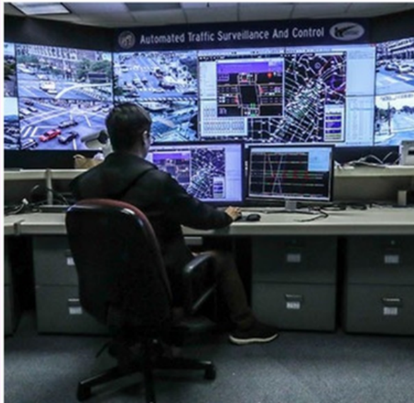
Automated Traffic Surveillance and Control (ATSAC) system monitors real-time traffic conditions in Los Angeles.
